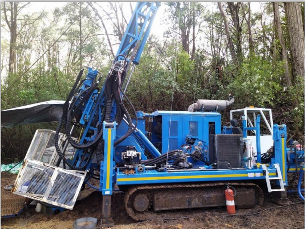
A large track mounted drill rig capable of drilling 1000m deep.
