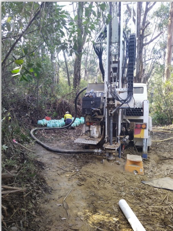
Percussion drilling rig with bagged samples in the background
